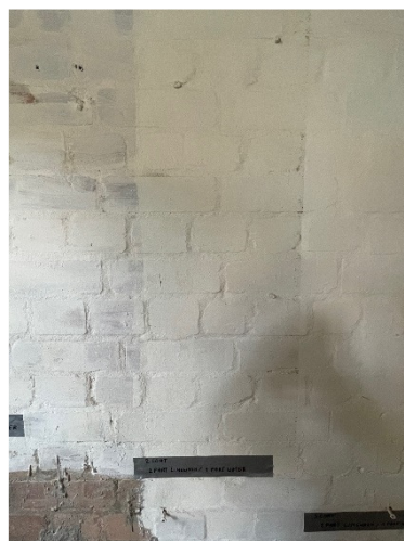
No 2: One-part Pozzolan Limewash one-part water plus one coat exterior limewash
