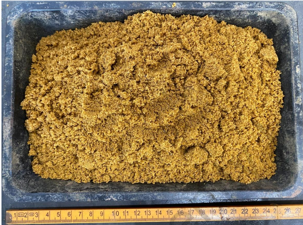
Plate 1: Washed Sand Subsoil Sample
