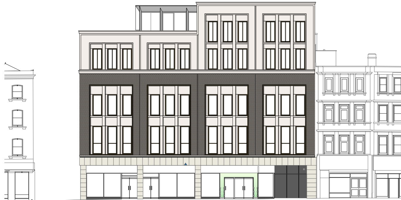
1. Retaining exiting brick piers with new 3rd and 4th floor extension above.
