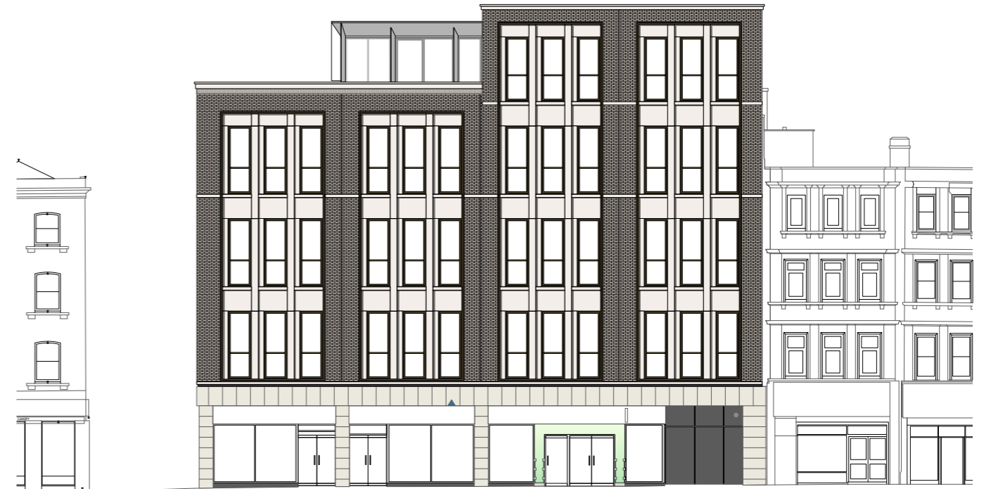
2. Retaining and extending existing brick piers to 3rd and 4th floor
