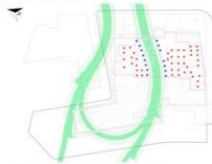
Figure 2.5 Museum Street core raft, movement-control and settlement-reducing pile layout at B2 level
