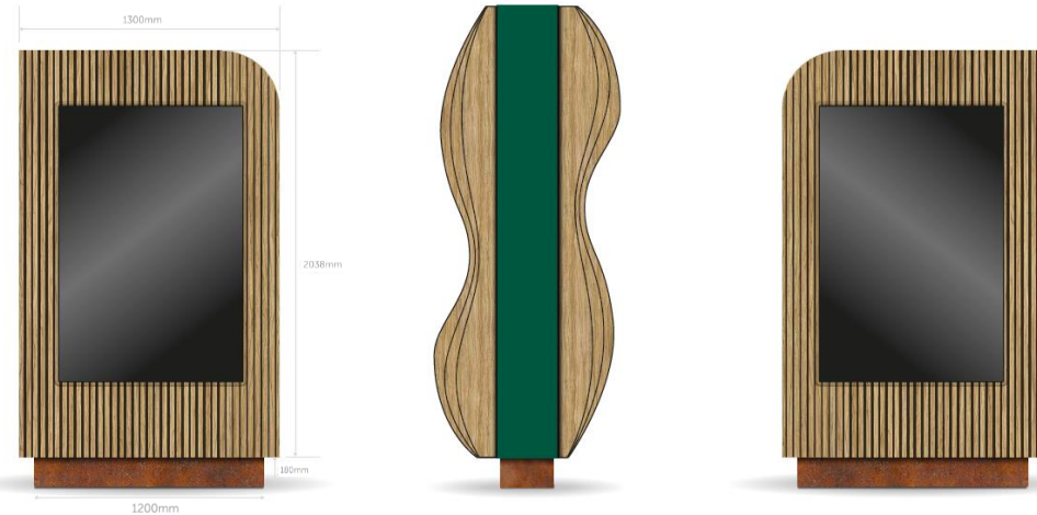
Timber slat parametric design to both faces with screen cut out. Brand green mild steel (or other more sustainable substrate) Steel corten kick plate.
