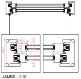
TIMBER SASH WINDOWS: All the windows are manufactured in hardwood including cills, fully weather sealed. The glazing is internally beaded with external rebate. All windows and doors to have trickle vent fitted into the window all to be according to latest building regulations. Apply 3 coats of sprayed applied microporous water based paint system. White matching existing.
