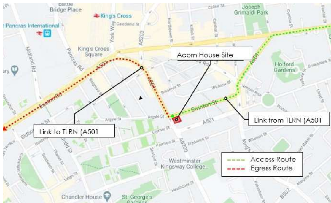
Figure 09 – HGV Construction Access and Egress Routes
