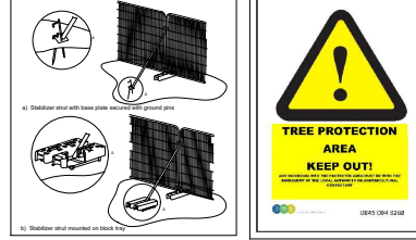
Figure 3. Examples of above-ground stabilising systems
