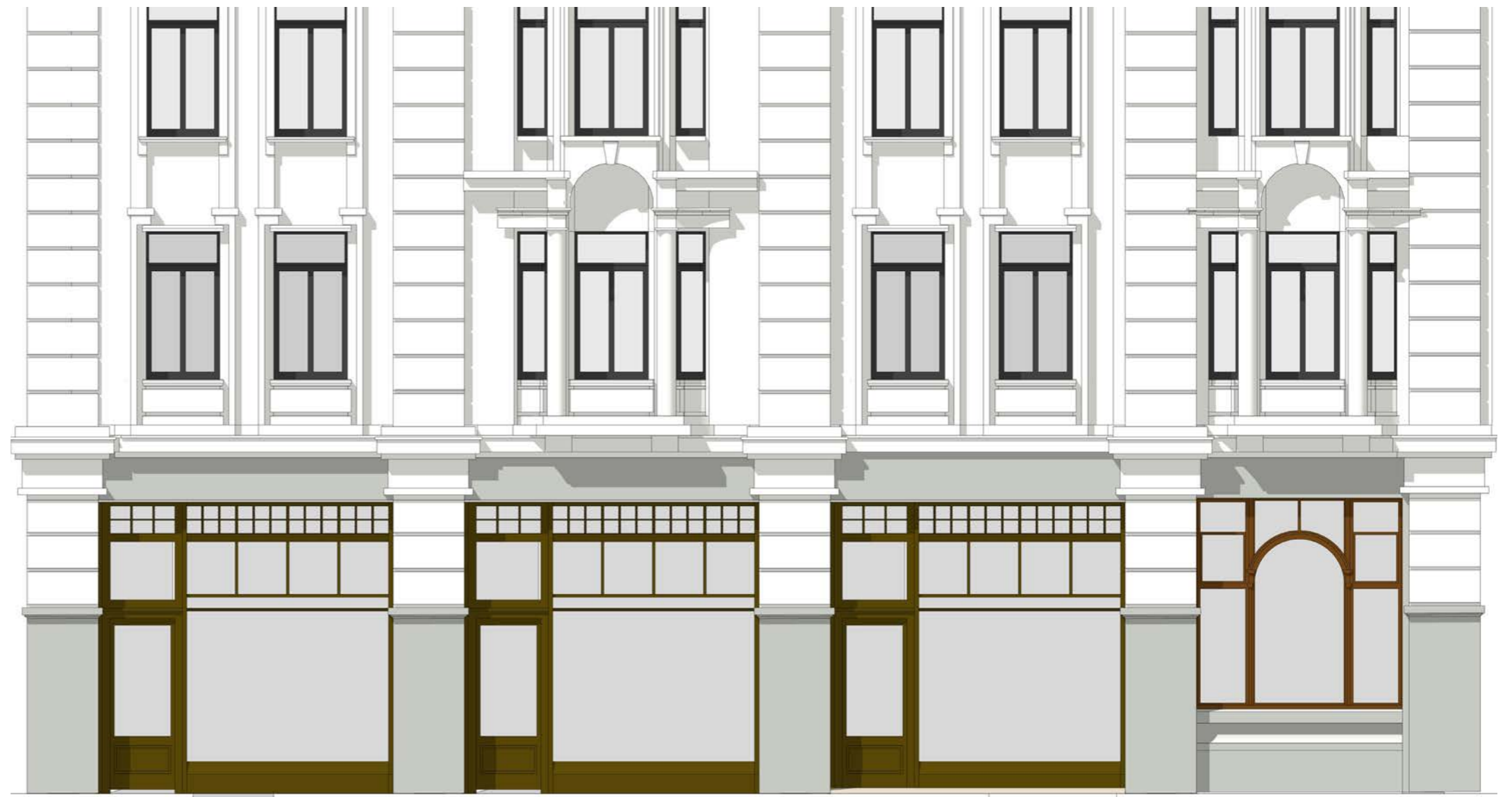
Figure 02 - Historic Edwardian 'Carter Seeds' shop front with Entrance door brought forward to be flush with the window bay
