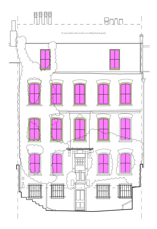
PROPOSED MAIN HOUSE SOUTH ELEVATION - PROPOSED WORKS TO EXISTING WINDOWS
