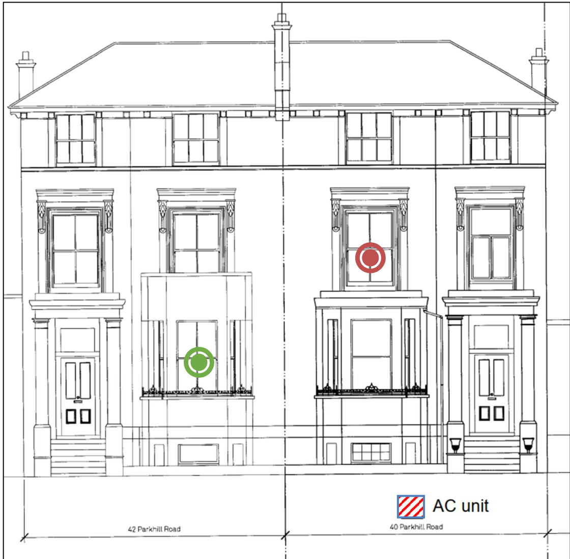
Figure 2.4 Site measurement position, identified receiver and proposed plant unit installation (Image Source: Paul Archer Design)
