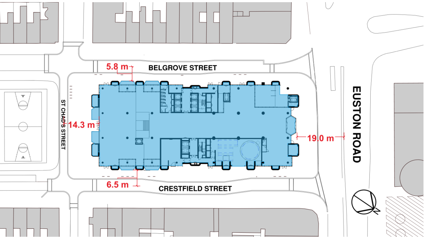
Figure 4: Site plan showing distances used for external fire spread assessment
