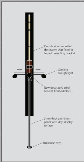
G. ONE x new aluminium bullnose trim Amenity Board panels, Powdercoated black, with face applied vinyl detail
