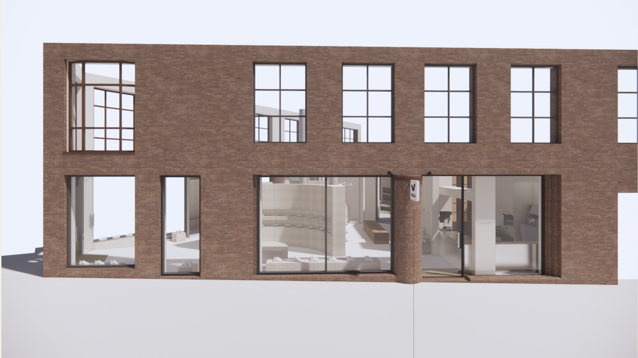
New non illuminated blad sign in powder coated metal with two supporting, discreet spots either side. Spots to be 3000k and powdercoated the same colour as the window reveals
