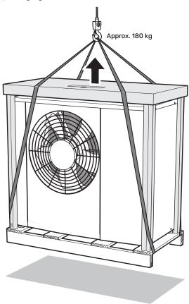
If S2125 needs to be transported across soft ground, such as a lawn, we recommend using a crane truck that can lift it to the installation location. When S2125 is lifted with a crane, the packaging must be untouched.
