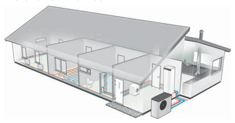
S2125 - a part of your climate system where S2125 is intended to be combined with one of the indoor modules VVM or the control modules SMO.
