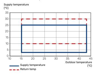
During shorter time it is allowed to have lower working temperatures on the water side, e.g. during start up.
