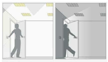
Absence Detection: Upon entering the room the person switches on the light as normal, but on leaving the detector switches off the lighting automatically. Lights can also be switched off manually.
