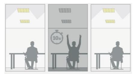
Absence Recovery: After an occupancy time out period has elapsed in absence mode, the unit temporarily enters a presence mode for 10 seconds allowing the occupants movement to bring the lights back on.
