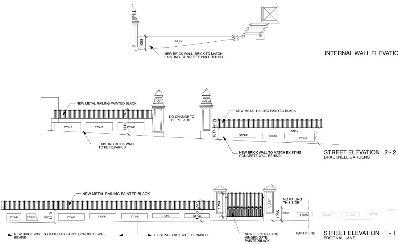
NOTE: ALL WALLS TO BE REBUILT TO EXISTING HEIGHTS
