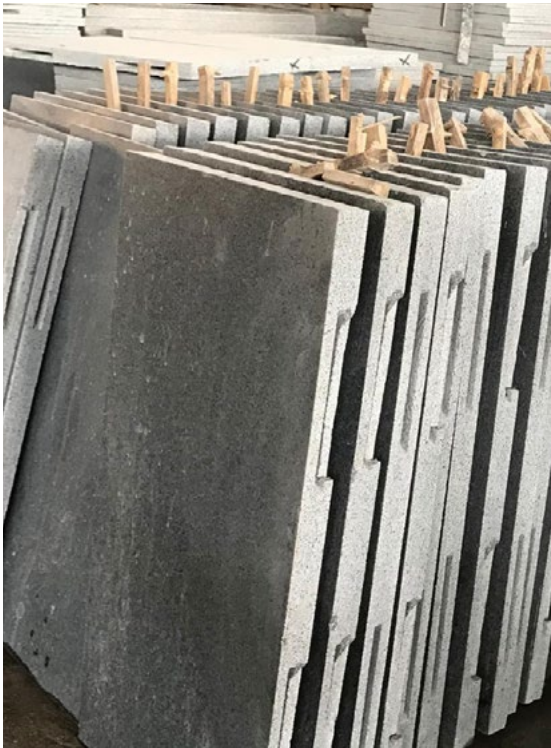
Cleaned and stored Granite sheets ready for reuse
