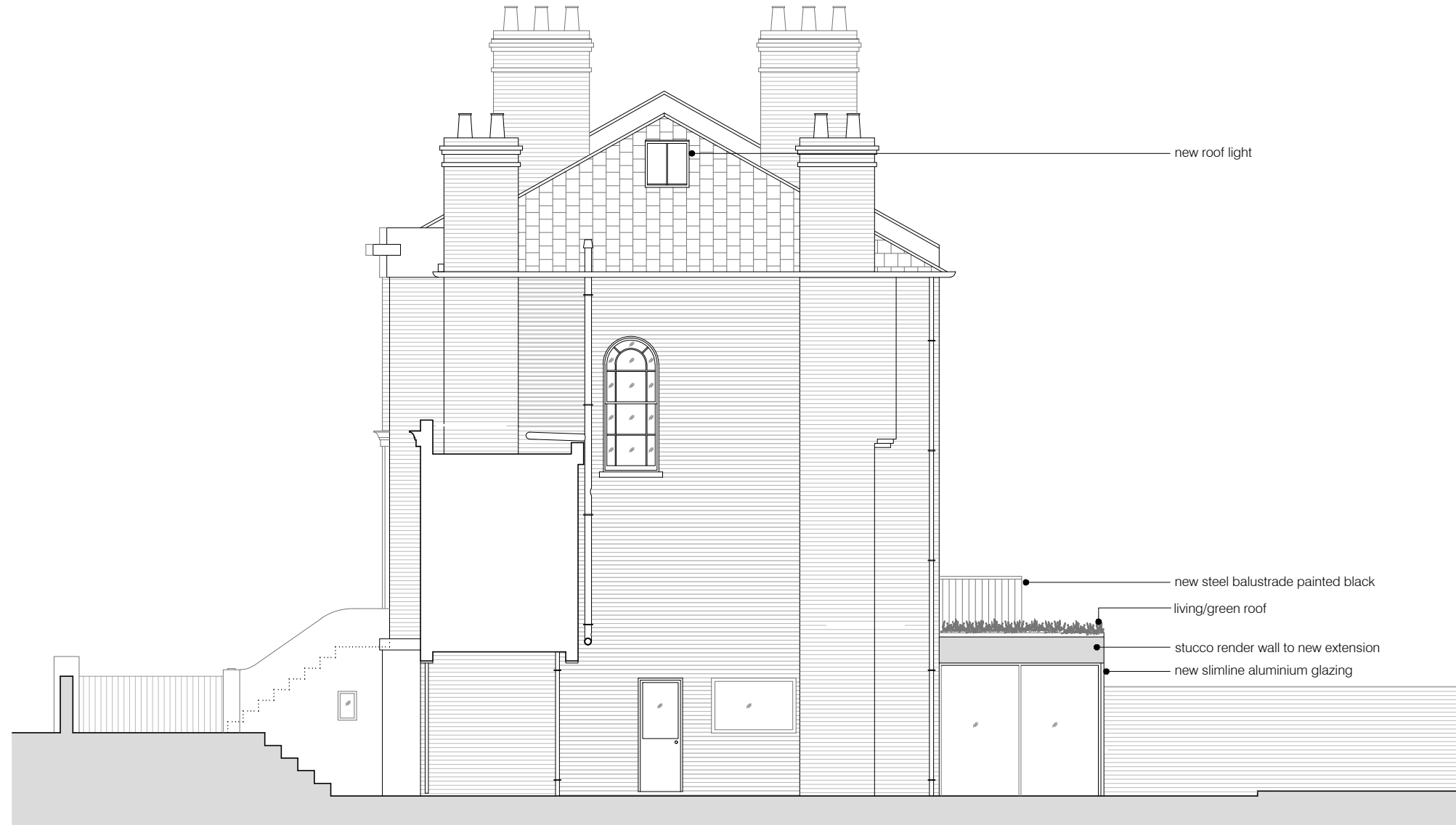
01 PROPOSED SIDE ELEVATION scale 1:100
