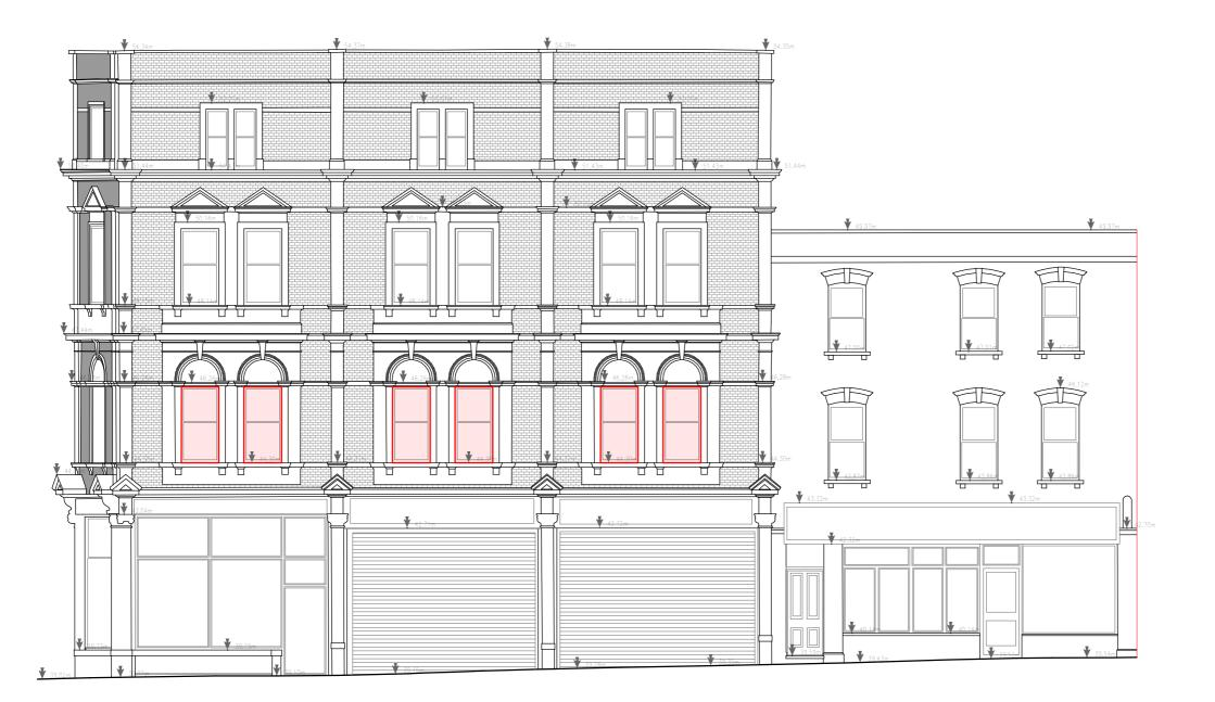
Highlighted windows to be replaced with new windows with the following characteristics:
