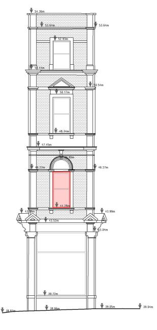
Highlighted windows to be replaced with new windows with the following characteristics:
