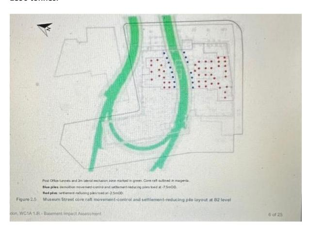
The engineering and construction challenges and associated risks described above, together with the need for the installation of the 1890 tonnes of piling would vanish if the option to **retrofit** the existing tower was pursued.
