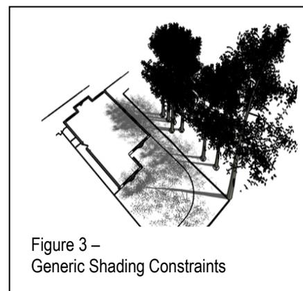
4.3.2 The shading constraints are crudely determined from BS5837 by drawing an arc from northwest to east of the stem base at a distance equal to the height of the tree, as shown in the diagram opposite. Shade is less of a constraint on non-residential developments, particularly where rooms are only ever temporarily occupied.
