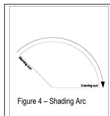
4.3.3 This arc (see Figure 4) represents the effects that a tree will have on layout through shade, based on shadow patterns of 1x tree height for a period May to Sept inclusive 10.00-18.00 hrs daily.
