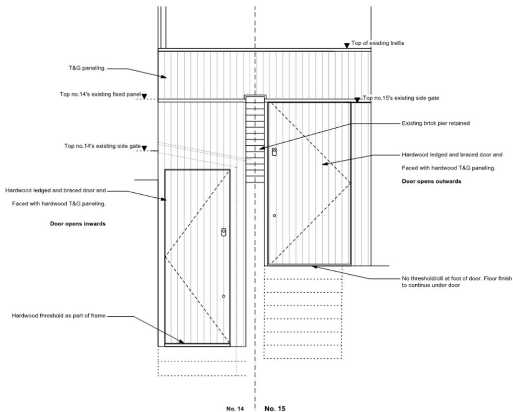
*Fig.1 Proposed Side gate drawing*
