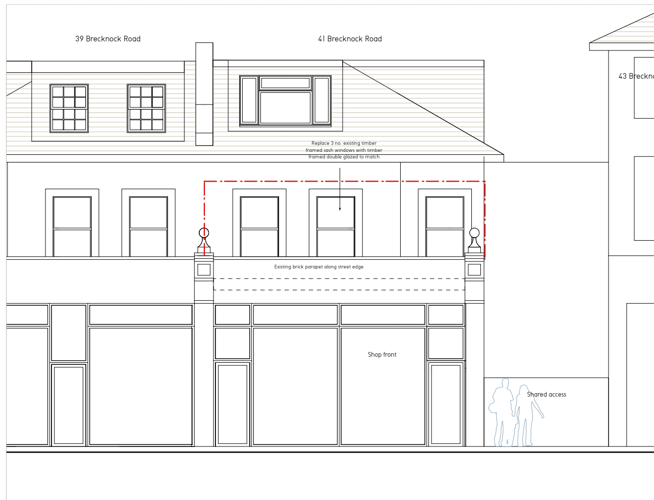
1 Existing North Elevation (Street)
