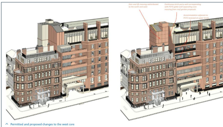
Figure 2: Permitted and proposed changes to the west core Provision of connection to the Paul O'Gorman (PO'G) building at each floor level
