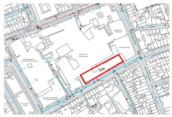
Figure 2.6 Water main pipes surrounding the proposed development
