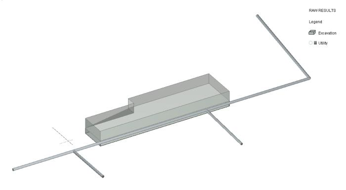
Figure 5.5 XDisp model geometry showing the utilities
