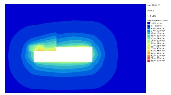
Figure 6.2 Vertical movement from Scenario B2 - CIRIA curves + LT loadings
