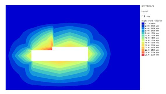
Figure 6.1 Horizontal movement from Scenario B2 - CIRIA curves + LT loadings
