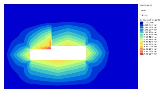
Figure 6.4 Horizontal movement from scenario B1 - CIRIA curves
