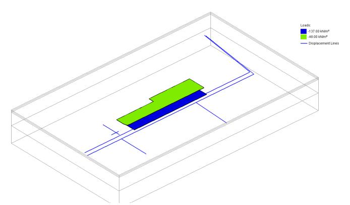
Figure 5.3 Loadings in Pdisp - ST Excavation + Demolition Heave
