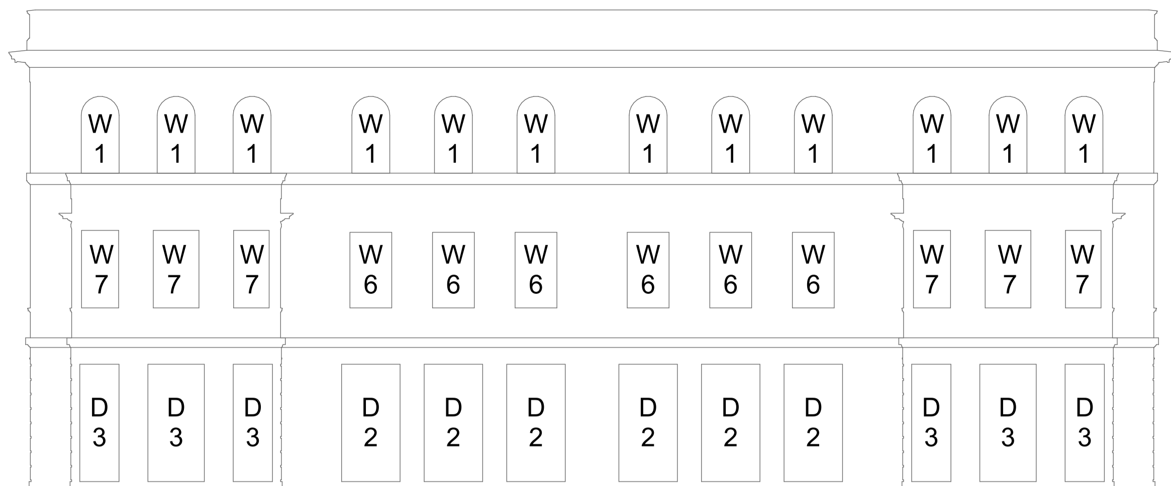
WEST BUILDING WEST ELEVATION
