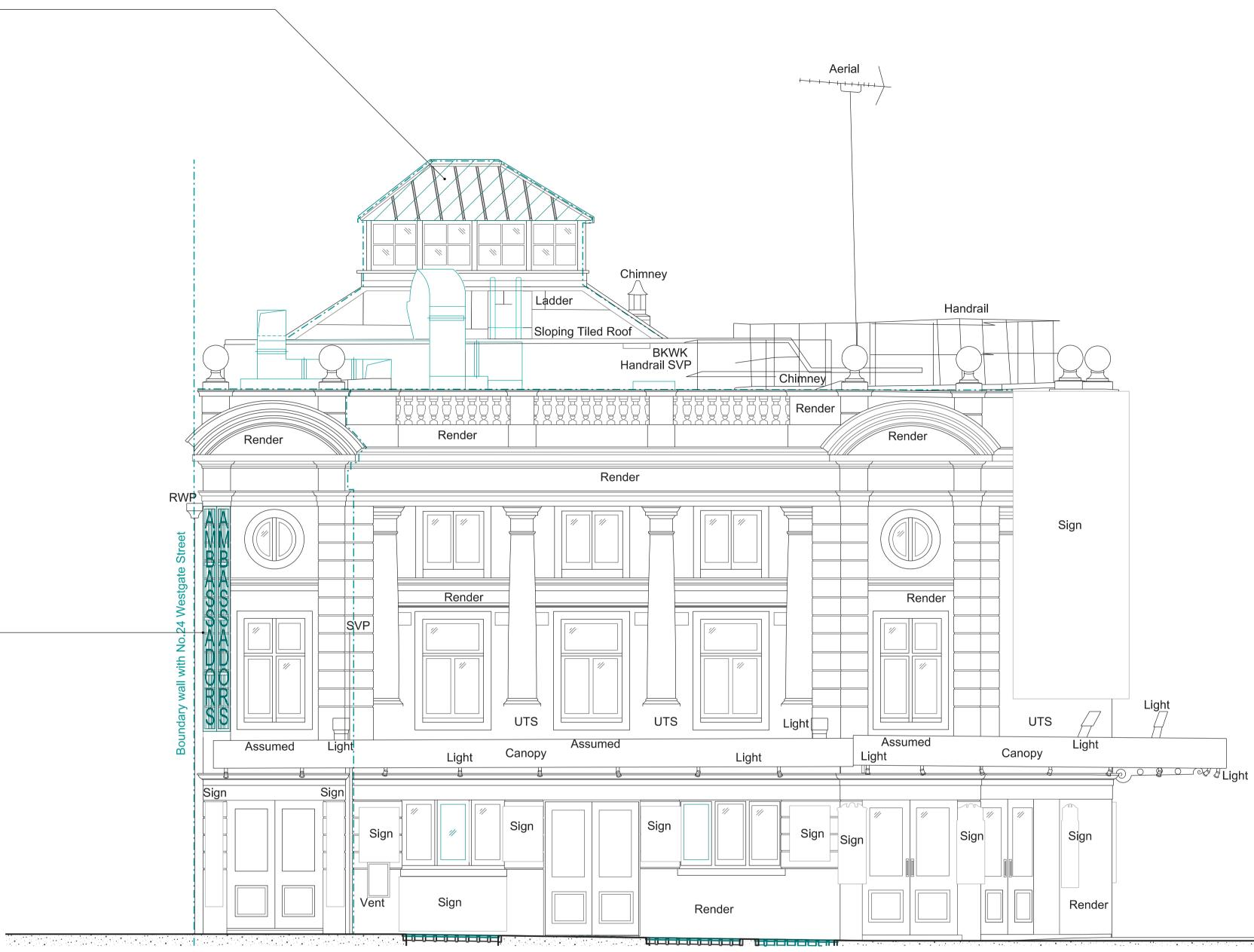
Note: works listed below have already been approved under the Planning and Listed Building Consent ref. 2022.3105.P and 2022.3599.L **Revised scope of lantern roof repairs** - 3no sides of the Lantern Roof have been patched a number of times and covered in a bitumen-like coating.
