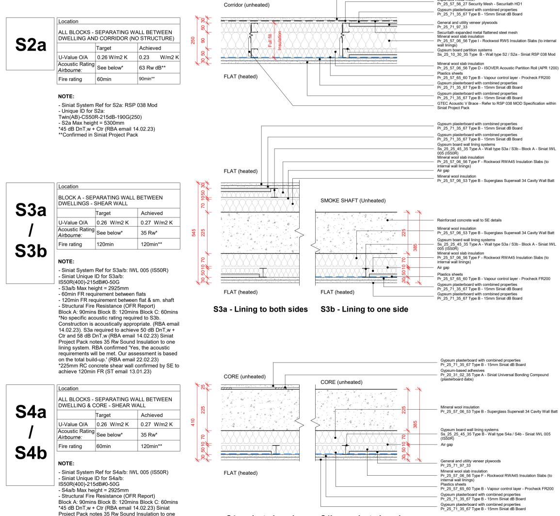
lining system. RBA confirmed 'Yes, the acoustic equirements will be met. Our assessment is based on the total build-up.' (RBA email 22.02.23) \*225mm RC concrete shear wall confirmed by SE to achieve 120min FR (ST email 13.01.23)
