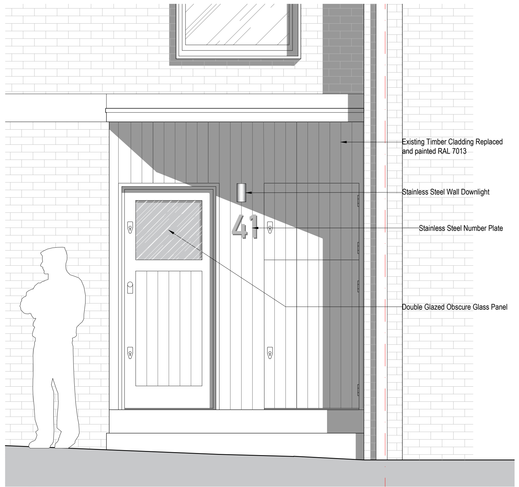
Proposed Rear Door and Panelling to No 41 Scale 1:20 @ A3
