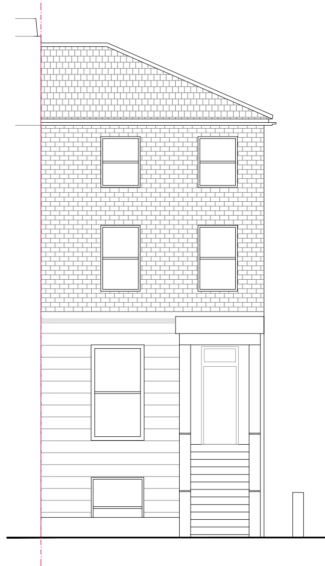
EXISTING FRONT ELEVATION
