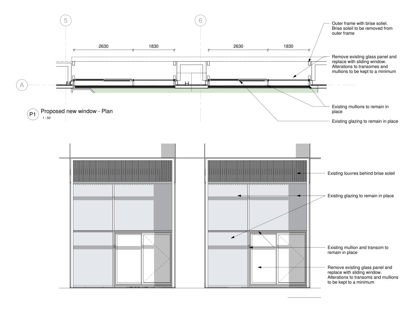
Existing outer frame supporting brise sloleil. Brise soleil to be removed from outer frame
