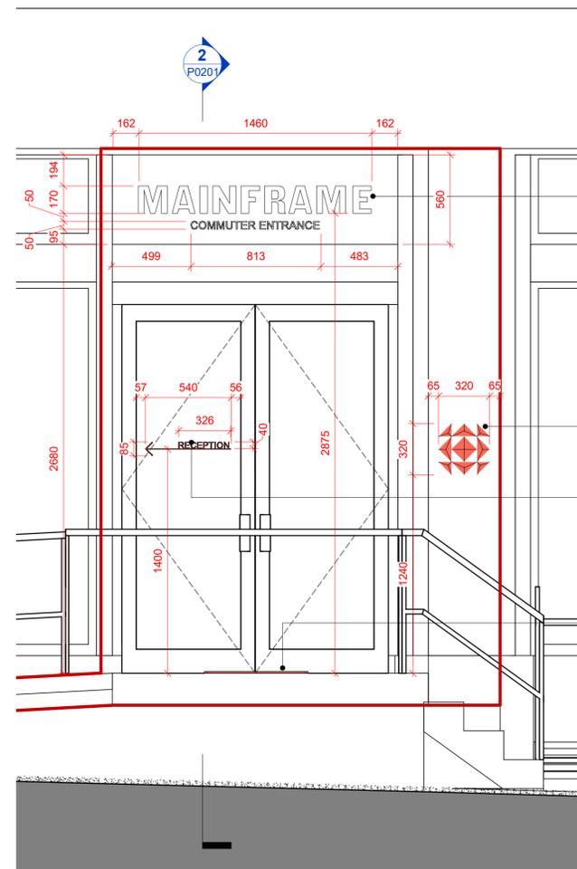
Building signage to be installed above secondary entrance door. Blank metal panel in RAL 7021 with "MAINFRAME" and "COMMUTER ENTRANCE" signage formed from individual lasercut metal letters in white finish with concealed fixings.
