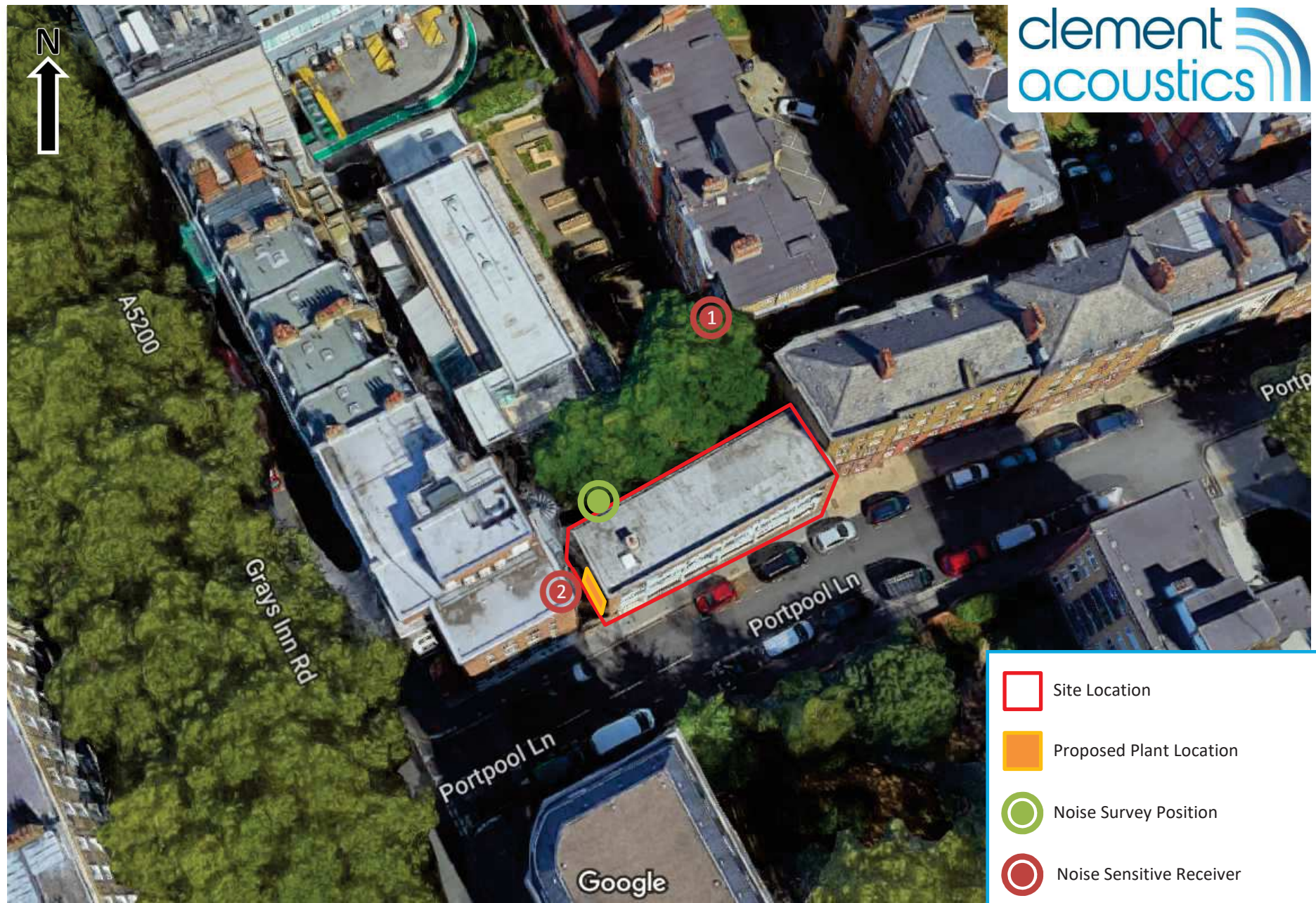
17935-SP1 Indicative site plan indicating noise monitoring position, proposed plant location and nearest noise sensitive receiver
