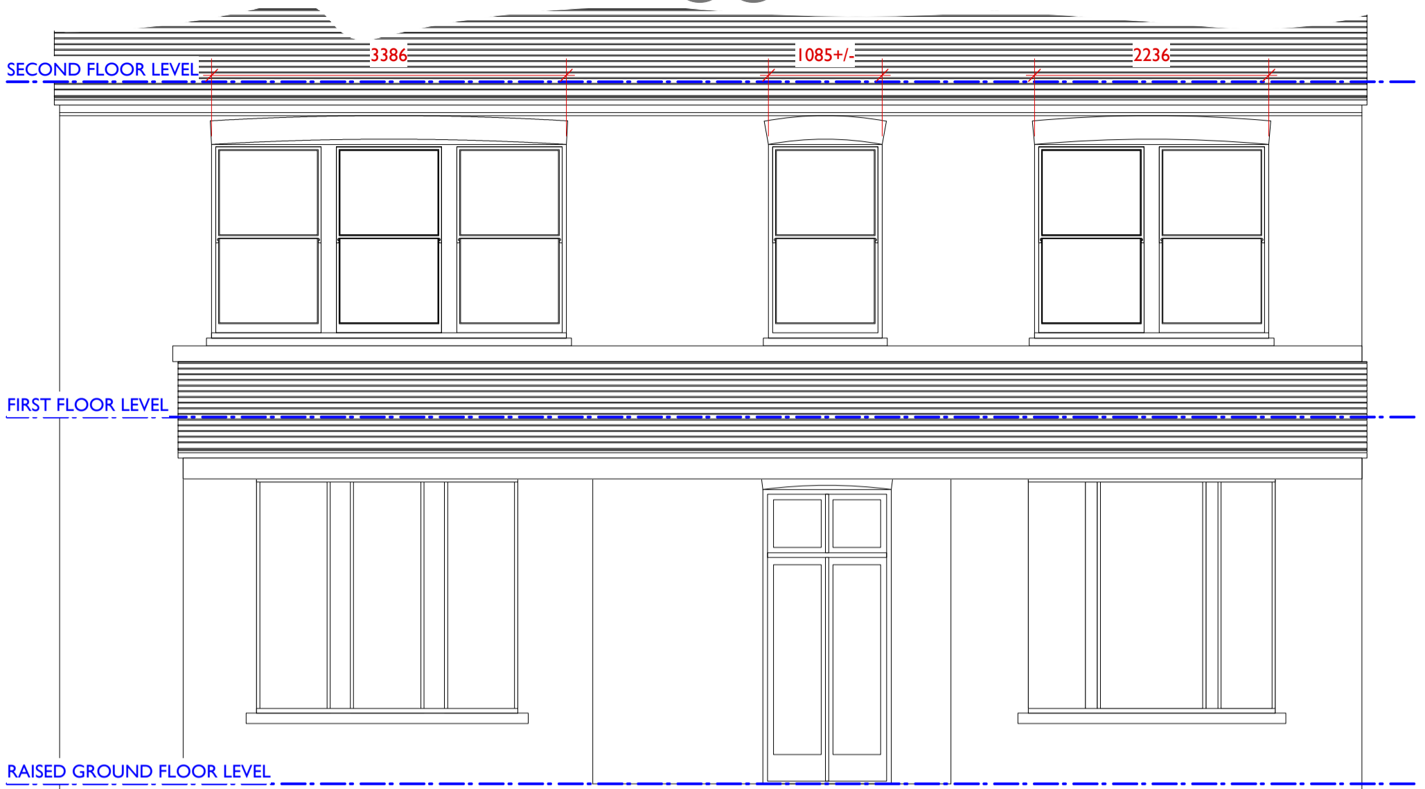
PROPOSED PART OUTLINE REAR ELEVATION - 3 BAY MASTER BEDROOM WINDOW & 2 BAY BATHROOM WINDOW
