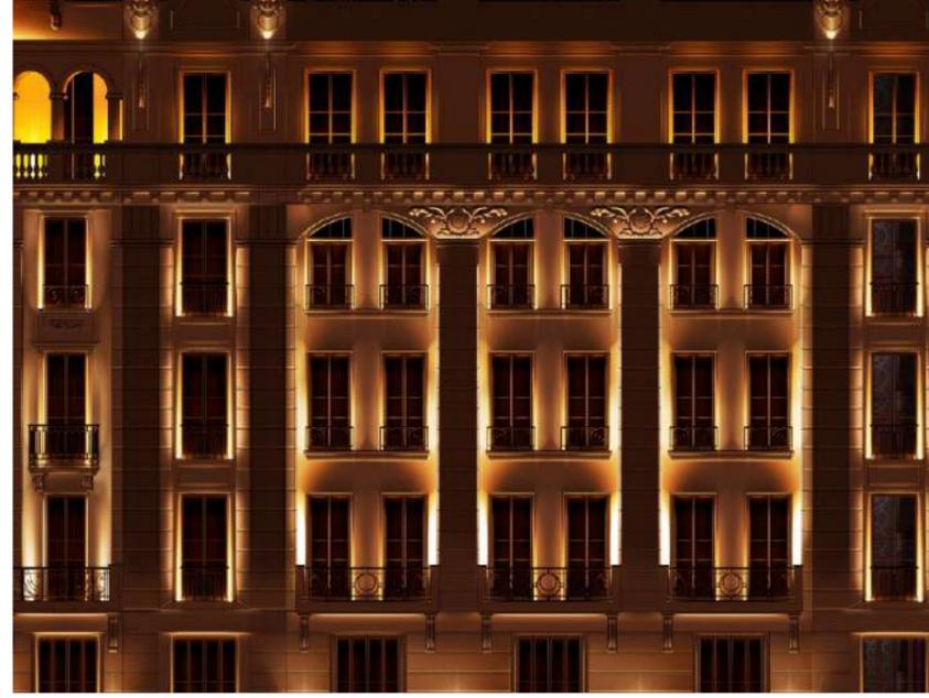
The existing façade lighting for Ambassadors Hotel is felt to be out of date. There is evidence of inefficient, high-powered fixtures being used. These fixtures have poor optical control causing a lot of unwanted light spill and high glare. Flood lights are used to ineffectively highlight signage and a few architectural elements.
