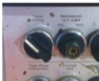
Photo - Forced inching mode - limited movement on drilling controls when gates are open
