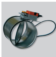
REMP Motorised damper, opens proportionately and is controlled by the BEAS control module. Power supply: 24 VAC or 24 VD, depending on the models.
