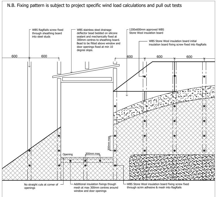
2 initial insulation board fixings required through each board, main fixings installed through scrim coat and mesh and in to RagRails at 300mm centres.
