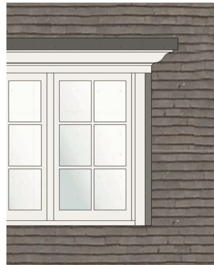
38 Frogнал concept of dormer with painted white timber decoration and lead cheeks and roof
