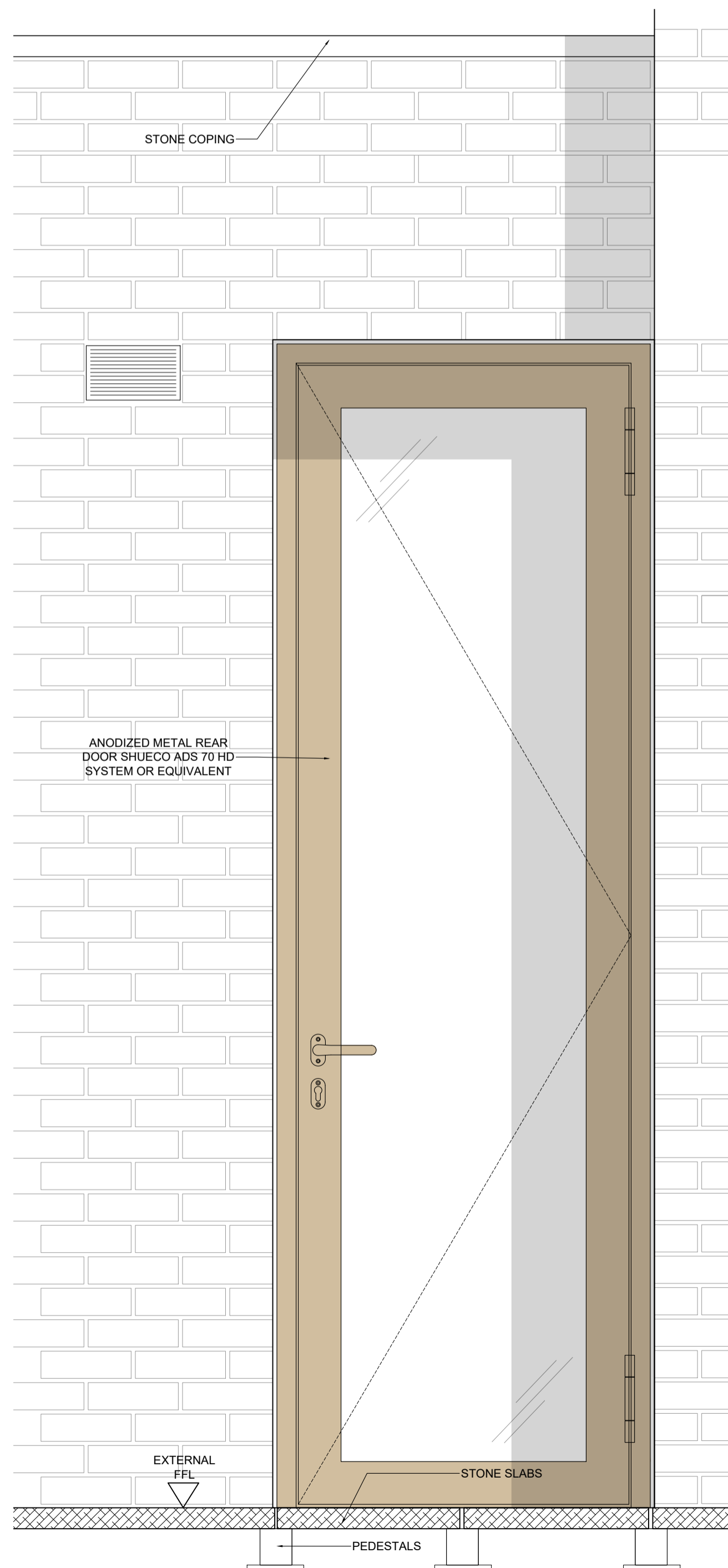
01 GROUND FLOOR REAR DOOR ELEVATION SCALE 1:10 @ A1
