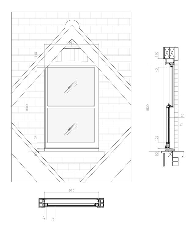
©1) PLAN, SECTION & ELEVATION - PROPOSED W1
