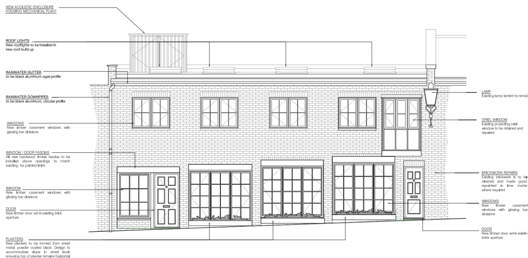
Proposed elevation showing the new acoustic enclosure, housing the mechanical plant.
