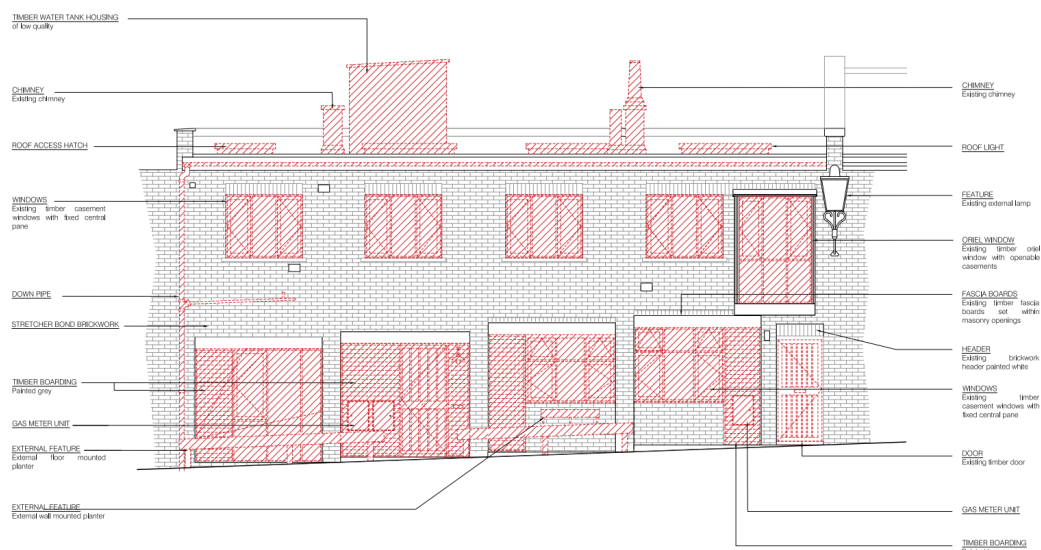
Existing elevation showing the timber water tank housing.
