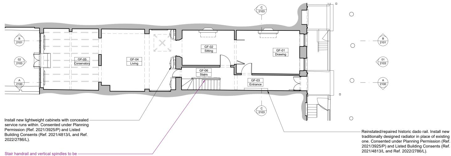
carefully stripped of existing modern paint. Timber handrail to be repaired, polished and stained. Vertical spindles to be redecorated
