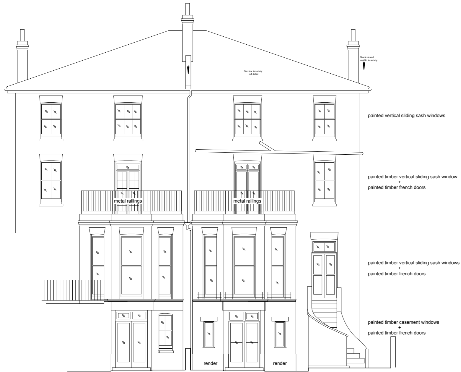
Existing Rear Elevation
