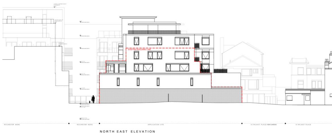
Above: Proposed North East Elevation (red line showing the existing building profile)
