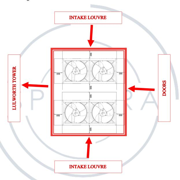
Doors will be opened at the opposite side by this means during the maintenance minimised noise will be transferred.
