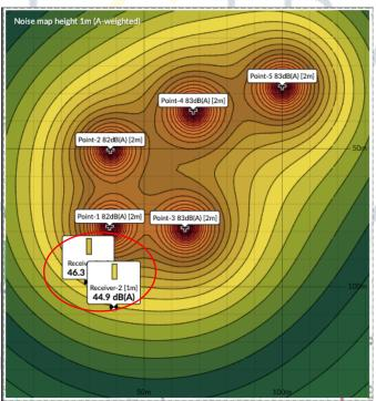
Critical Noise Levels are higher than requested at the Lulworth Tower façade without using any enclosures. (Reciever-1=46.3 dB(A), Reciever-2=44.9 dB(A)
