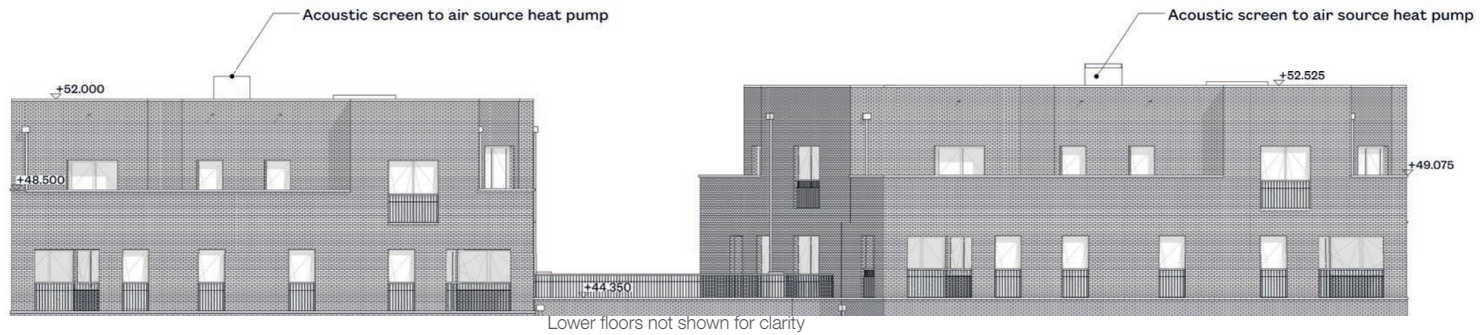
ASHPs and enclosure - Approved October 2020 East Elevation
