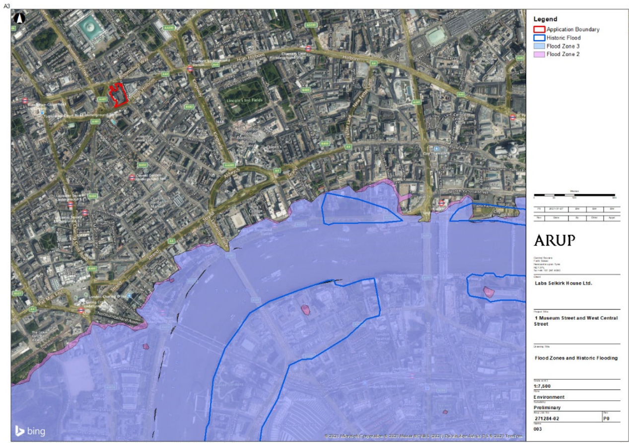
Figure 5: The River Thames has flood defences along its banks, protecting the application site from 1 in 1000 year tidal flood events.
