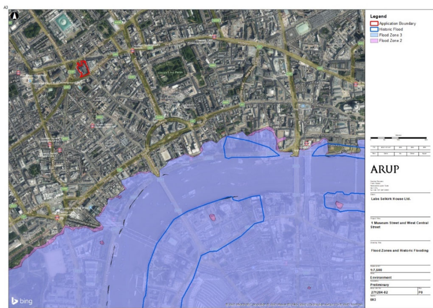
Figure 3: The Council's SFRA mapping showing the application site situated outside of Local Flood Risk Zones 15 and historic flooding areas.
