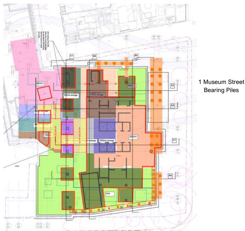
Figure 2 Locations of the proposed bearing piles outside of the basement footprint
